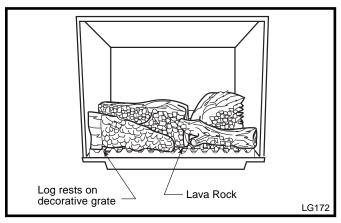
Fig. 24 Completed log installation.
